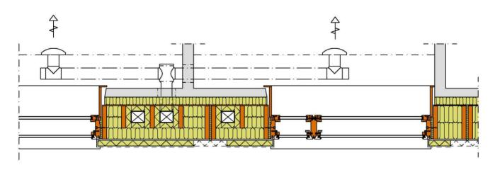
Fig. 4 The vertical ventilation ducts for the supply air are installed in the elements.
