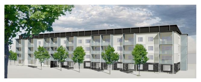
Fig. 5 The new façade materials are plaster rendering, cement fibre board (day-care centre) and wood cladding (balconies). The 3-dimensional surface of the plaster rendered facade and the variation of colour show the division of apartments behind the façade. The target of the architectural design was to upgrade the facades, but still maintain a connection to the original character of the building. Image: Kimmo Lylykangas Architects.
